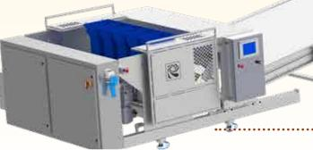
**Dough Handling** The completely automated Dough Handling System precisely portions, conditions and transports dough to the Low Pressure Extruder.
