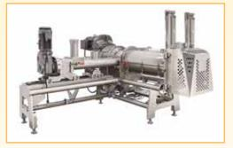
The EX Continuous Mixer produces low absorption dough for products such as pretzels, bagels, cookies and crackers.
