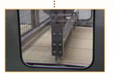
**Guillotine Cutting** The single-blade design provides precise, consistent cutting and product separation of sticks and nuggets across the width of the line.
