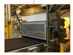
Sheeting The process begins with a primary Sheeter producing a hole-free sheet at a uniform density, which is critical to automated packaging systems after the oven.
