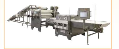
**Dough Handling** The dough transport conveyor ensures that the dough makes it from the mixer to the 2-Roll Sheeter hopper on a first-in, first-out basis
