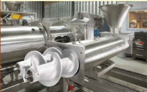
Preblender shown rotated for cleaning purposes
