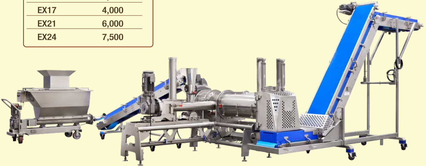
Exact also offers automated dough handling systems to transport dough to downstream equipment.
