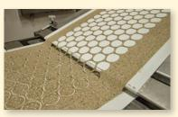
L. Green sheeting line consists of a 3-Roll and 4-Roll Primary Sheeter, two Gauging Stations, and a 2-station Rotary Cutter. Simple sheeted products can be made on a 2-Roll Sheeter.
