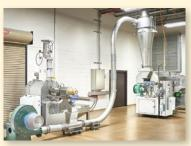
A single screw extrusion system is also available for producing expanded snacks from corn, rice and other cereal ingredients. The system includes a Dry Ingredient Ribbon Blender, High
