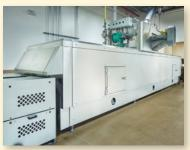
For traditional cookie products, we have a full production line that includes a Thomas L. Green Rotary Moulder and Wirecut Machine. The 600mm wide line also includes a single zone, 9m long PRISM Emithermic Oven that includes both radiant and convective heat transfer methods. The PRISM OVEN features our Thermatec High Radiant Panels that ensure a consistent, uniform bake by storing and reradiating heat to the product. The line is controlled from a touch screen Operator Interface Terminal.
