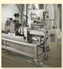
and mass flow liquid feed systems, in order to consistently deliver ingredients and validate the process for scale-up. Line outputs are approximately 20-90 kg/hour and are accommodated by either continuous or batch mixing.
