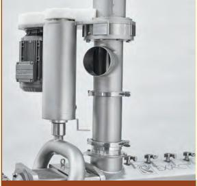
Ingredients are fed directly into the Hydrobond unit and mixed together before entering the mixing chamber.
