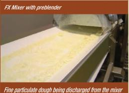
The **FX Continuous Mixer** is designed to distribute small amounts of moisture evenly into large amounts of powder. This is accomplished by lifting the powder into atomized liquids. This mixer is ideal for hydroscopic powders such as potato flakes used to make fabricated potato chips or any other low moisture mixtures.
