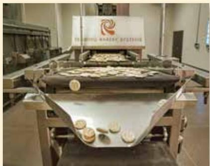
After baking, the product is transferred into a single zone, 4.8 m long x 600 mm wide forced convection dryer. The PRISM Oven and Dryer are individually controlled using a remote OIT control station.
