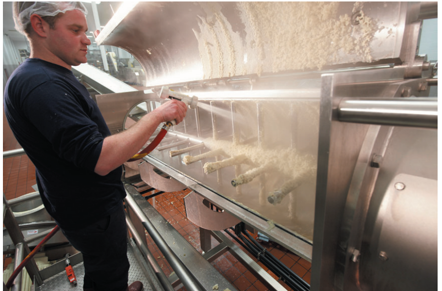
▲ Sanitary design of the continuous mixer allows full access to internal parts and mechanisms.
