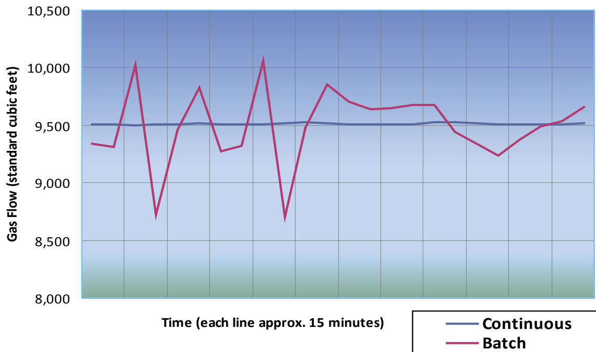
Figure 1: A gas flow meter was used to measure the gas demand on an oven baking crackers. Four hours of data was recorded while the oven was supplied with batched dough and depicted above in red. Data supplied during a similar time period for continuously mixed dough supplied to the same oven is depicted in blue.
