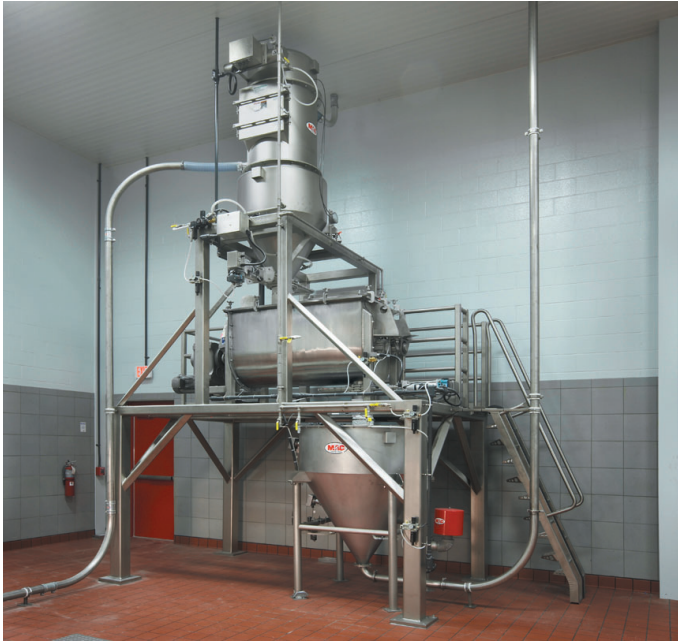
▲ This preblending system combines micro and minor ingredients that are then pneumatically metered to the continuous mixer.
